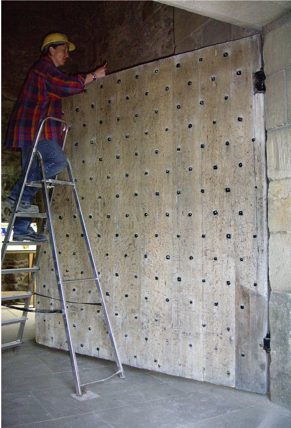
ILLUS 6 Sampling in progress on the massive oak door leading from the Inner Close into the Palace at Stirling Castle. This was made from Eastern Baltic oak boards some time after 1533
