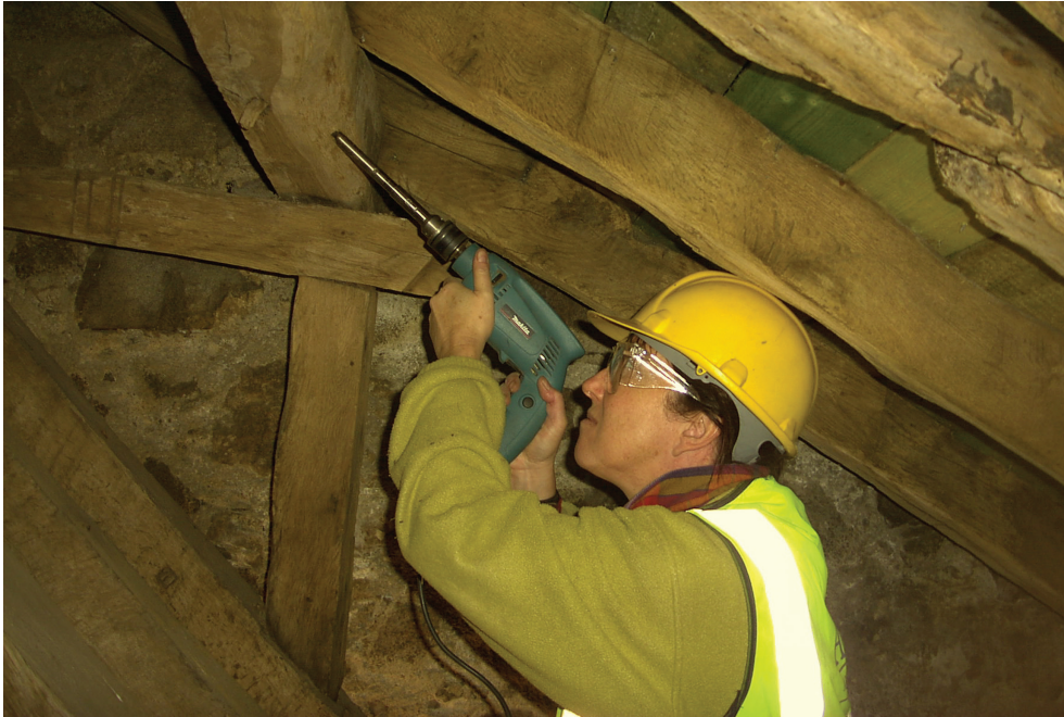
ILLUS 9 Sampling of the early 17th-century roof of the mansion house, Drum Castle. The knottiness and wavy grain of the locally grown oak is visible on the rafters above and behind the dendrochronologist
