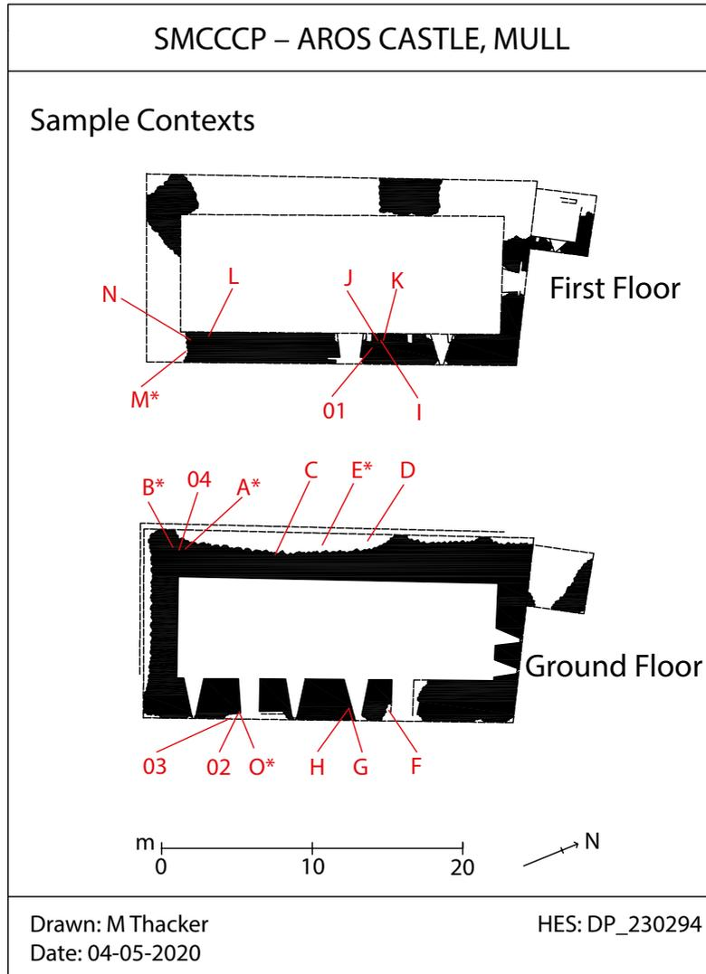
ILLUS 4 Ground-floor and first-floor plan drawings of the north-west block at Aros Castle with in-situ sample location measurements plotted. Sample codes have the ACM prefix removed and those marked with an asterisk represent MERLF fragments selected for radiocarbon analysis. (Plan drawings after RCAHMS 1980 DP\_230294 © Crown Copyright: HES)
