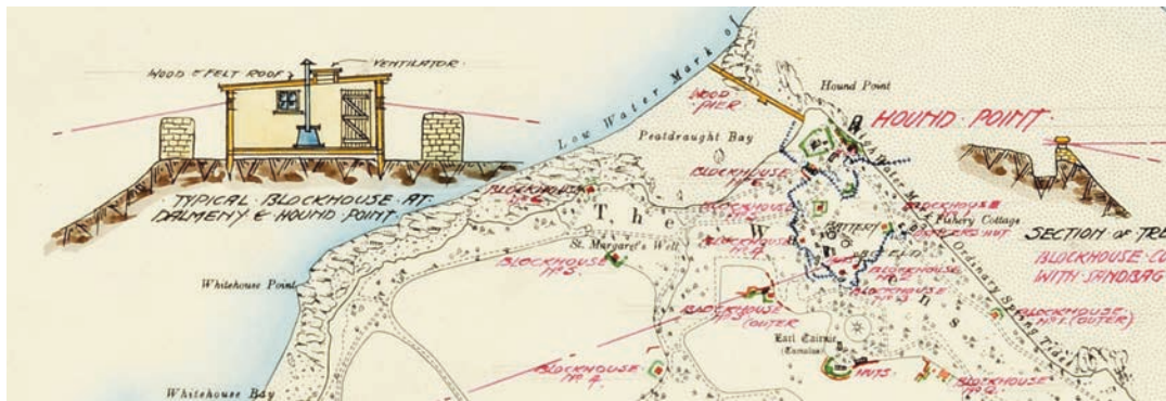
ILLUS 25 Map extract showing the defences round the Hound Point Battery, and the cross-section of a blockhouse (TNA WO 78/4396 1916)
