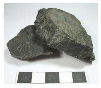
Illus 9 Aphyric pitchstone from Dun Fionn, Corriegills (GLAHM 134054). The pitchstone shows faint flow-banding on weathered surfaces. The pale spots on broken surfaces are small spherulites.
