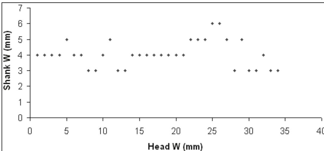
Scatter diagram showing the dimensions of nails: head width (x-axis) vs shank width (y-axis) in mm.
