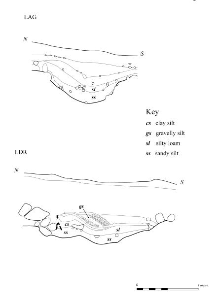
Illus 4.14 Sections of ditches associated with the Phase 1 bypass road in Area L
