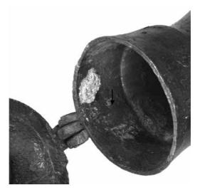
ILLUS 3 The vertical seam (arrowed)
